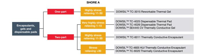
Thermally conductive encapsulants, gels and dispensable thermal pads
