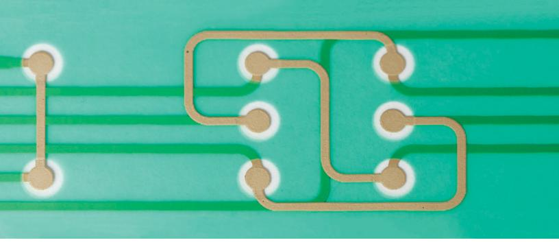
**Dielectric** – Non-conductive, dielectric inks insulate multilayer circuitry to allow for circuitry crossover and multilayer applications. These materials offer excellent flexibility, humidity resistance and additional protection for improved strength and performance for multiple applications including keyboards, copper-etched circuitry and hybrid circuits.
