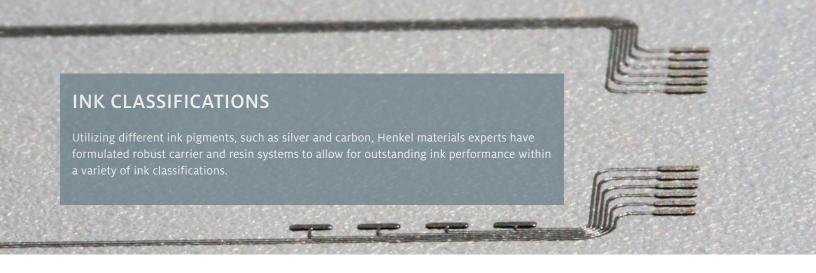
**Silver** – Silver is the most electrically and thermally conductive of all metals and is used as the basis for many of Henkel's conductive ink products. When combined with specific resin systems, Henkel silver inks can deliver better flexibility, crease resistance and longevity. These inks find uses in many different applications within numerous market sectors and are available in UV and solvent formulations.
