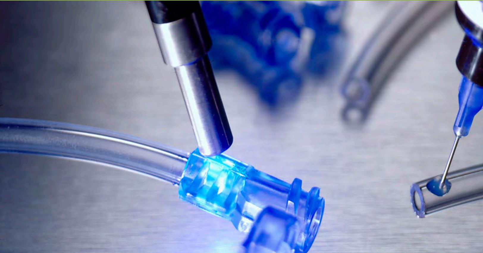
For more than 35 years, light-curing technology has allowed manufacturers to lower processing costs, produce higher quality products, and eliminate the use of harmful chemicals from the workplace. First introduced in the early 1980s for ink and thin coating applications, the technology has advanced tremendously over the last three decades, becoming the method of choice for many other industrial bonding, sealing, coating, potting, and tacking applications.
